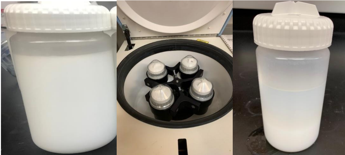
Fig. 6 The material is placed in centrifugation containers (left) and centrifuged (center). The result is the separation of the gel from the liquid (right).
