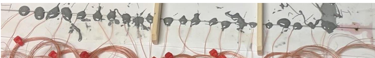
Fig. 3 The array of thermocouples glued to the microchannel with high-thermal-conductivity glue is shown.
