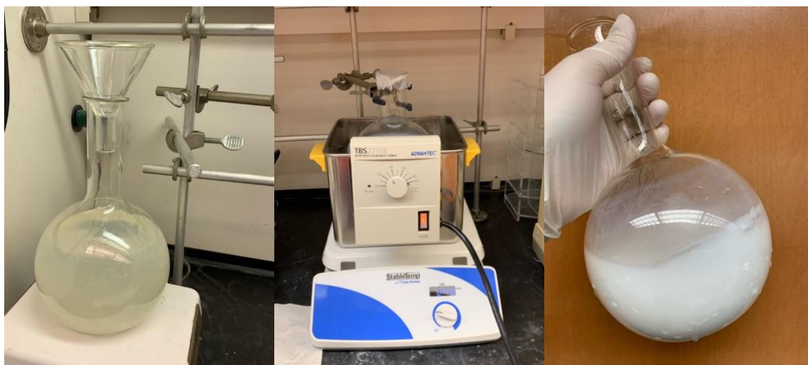
Fig. 5 The reaction mixture is prepared in a flask (left) and placed in a water bath (center). After 4 days of stirring, the mixture becomes white and gel-like (right).
