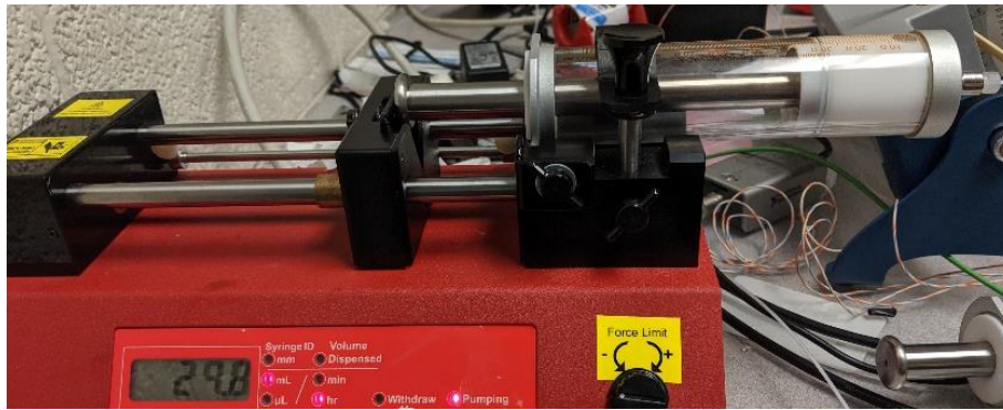
Fig. 4 A syringe is mounted into the syringe pump to allow nanofluid to flow through the system. The syringe is shown loaded with TiO 2 nanofluid.
